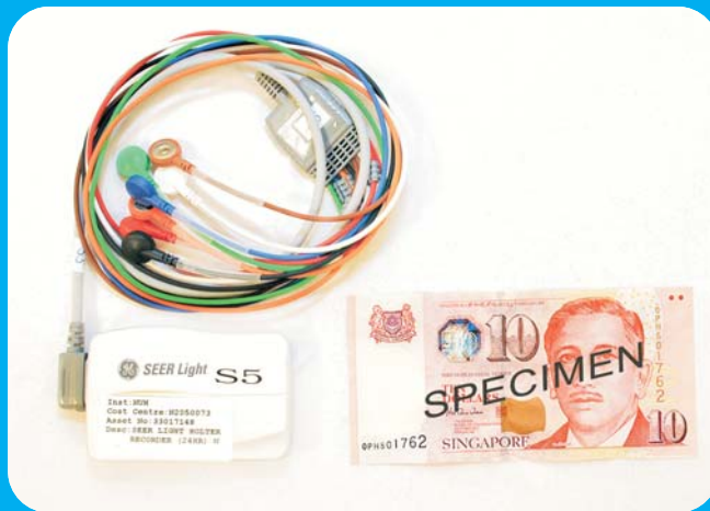
An ambulatory ECG recorder with a ten dollar note for size comparison.
