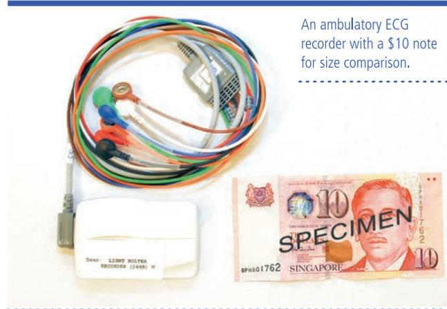
An ambulatory ECG recorder with a \$10 note for size comparison.
